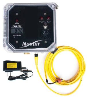
This Pro CO Alarm Analyzer combines carbon monoxide detection, a low pressure alarm, an external high temperature sensor and a low pressure flow meter / regulator. Components are mounted in a water and impact resistant case with a clear cover that is compatible with outdoor and marine environments. Available in two power options.
