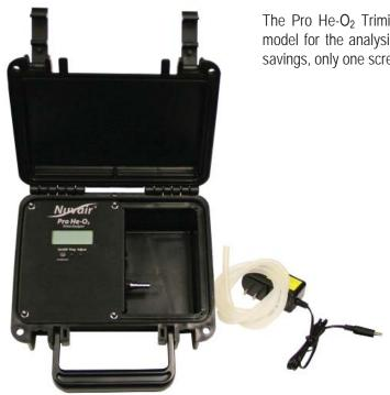
The Pro He- $O_2$  Trimix Alarm Analyzer represents the most economical and contemporary model for the analysis of oxygen and helium in mixed gas with nitrogen. For an added cost savings, only one screen is used to cycle between He and  $O_2$  readings.
