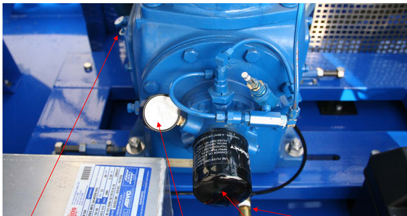
Compressor Oil Fill & Dip Stick
