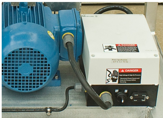
Electric Motor Power Switch and Tach.
