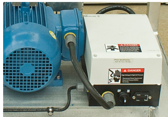
Electric Motor Power Switch and Tach.
