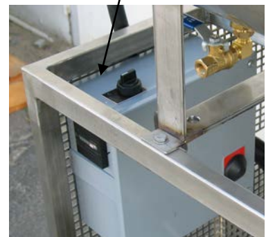
On/Off LP Feed Air Supply Valve Handle in Open Position
