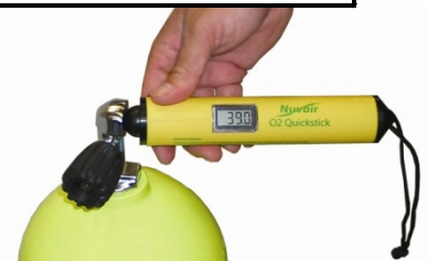
Use Independent Oxygen Analyzer for Verification
