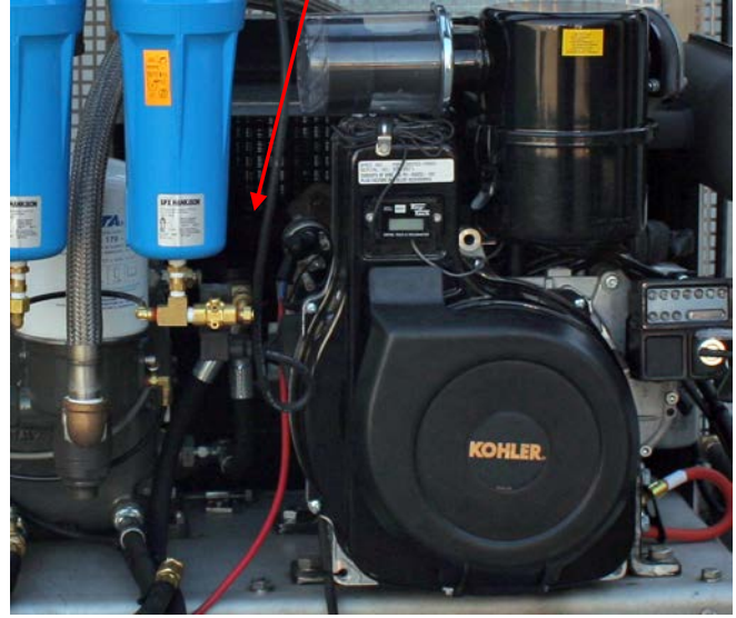
Oil Filter for LP Compressor
