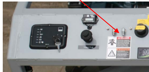
Fill Whip connection points on compressor
