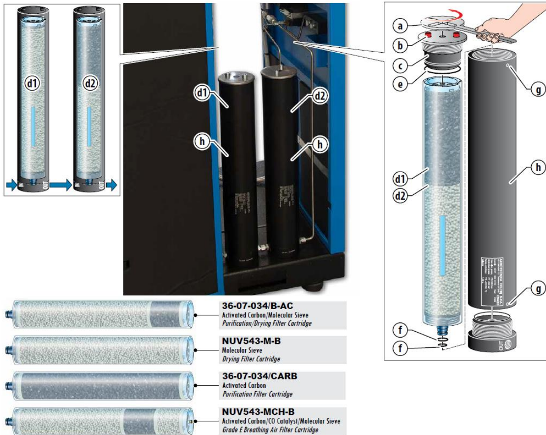
Figure 29. Air filter changing diagram.
