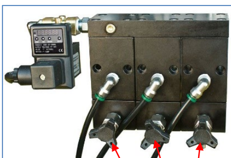
Auto Drain Manual Bleed Valves
