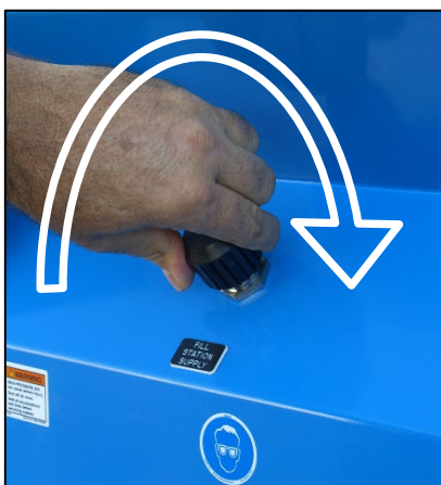
Step 10: Open fill station valve.
