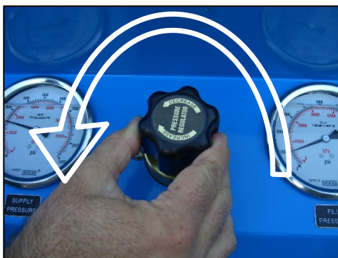
Step 2: Turn HP to HP regulator counterclockwise (decrease).
