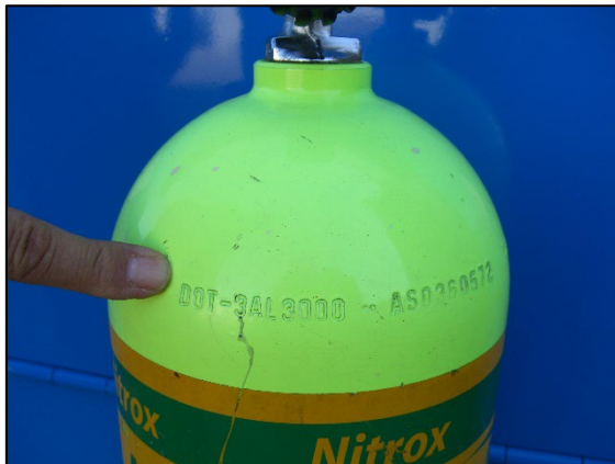
Step 4: Check cylinder for proper rating valid test date, and maximum fill pressure.
