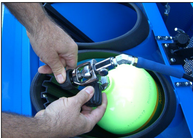
Step 8: Open cylinder valve.
