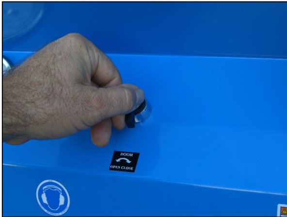
Step 14: Open fill station door.
