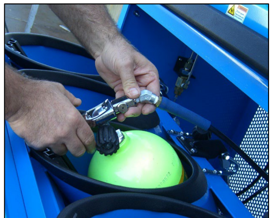
Step 17: Remove fill whip from cylinder.
