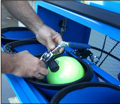
Step 6: Connect fill whip to cylinder.
