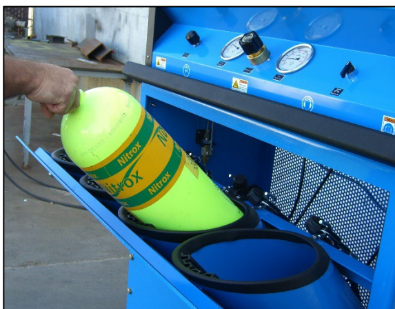
Step 18: Remove cylinder from compartment.
