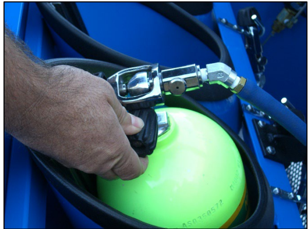
Step 15: Close cylinder valve.
