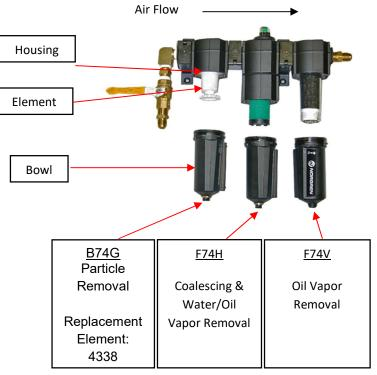
Inspect Elements for any unusual degradation or wetness. Element degradation can indicate more serious problems. Contact Nuvair for assistance.
