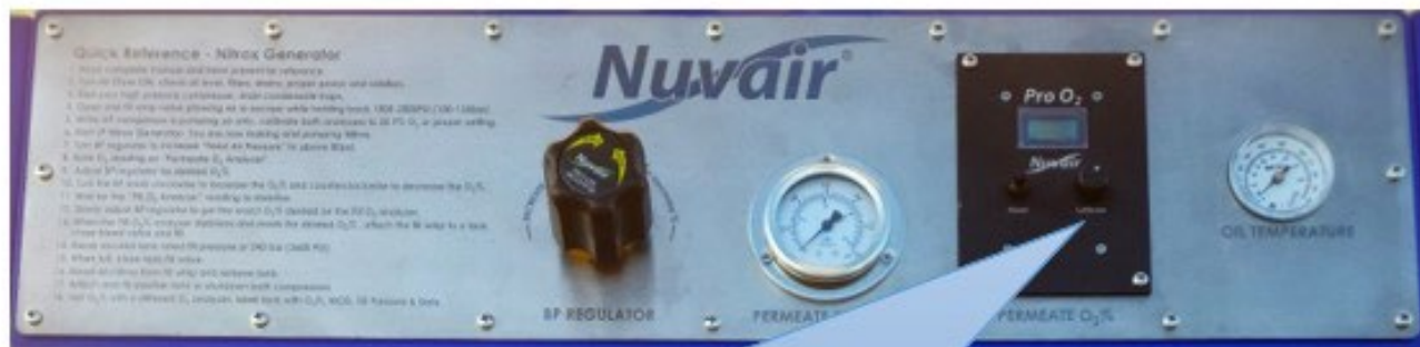
Pro O 2 Analyzer Calibration Knob Inline Oxygen Analyzer Provides Rough Estimate of Oxygen Content
