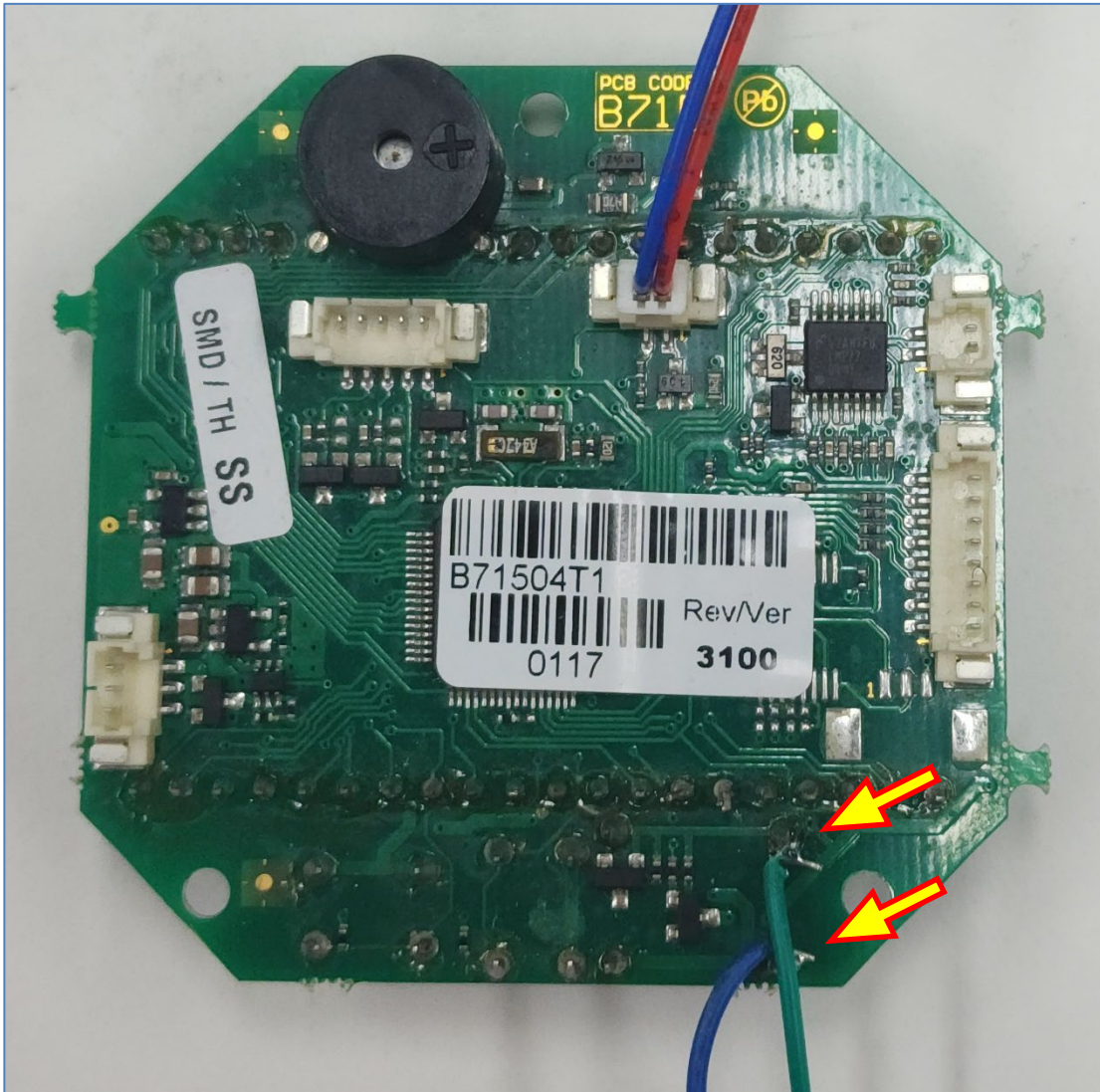
Step 3: Solder green and blue “switch” (SW) wires onto Pro Analyzer circuit board.
