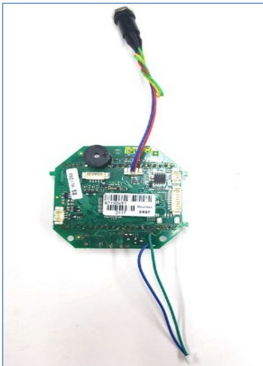
Step 1: Gain access to the Pro Analyzer enclosure and remove Pro Analyzer circuit board (pictured).
