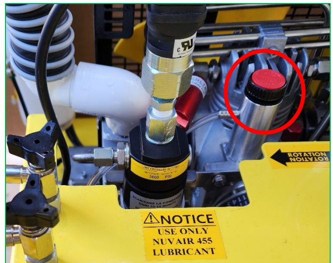
Figure 14. HP compressor lubricant fill tube.
