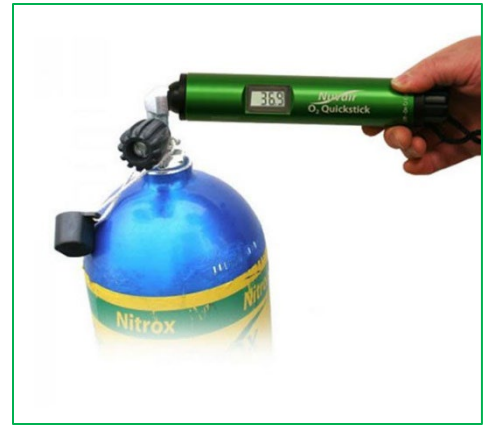
Figure 12. Use independent oxygen analyzer for verification.
