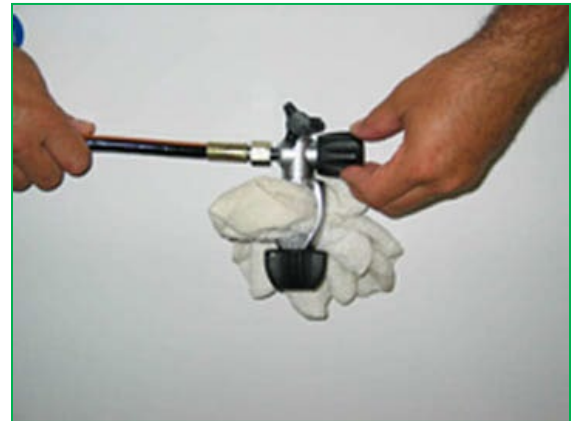
Figure 6. Adjust fill whip to maintain pressure. Insert a clean rag in fill whip yoke for sound muffling.
