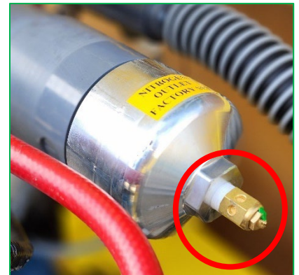
Figure 2. Fixed factory set nitrogen discharge outlet.
