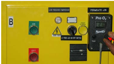
Permeate Oxygen Analyzer Provides Rough Reading
