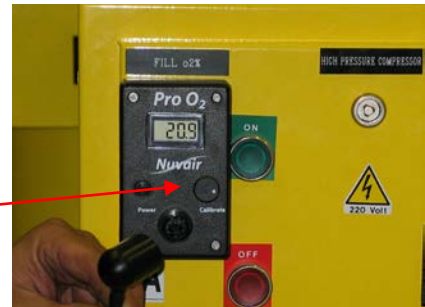
Fill Oxygen Analyzer Provides Precise Reading
